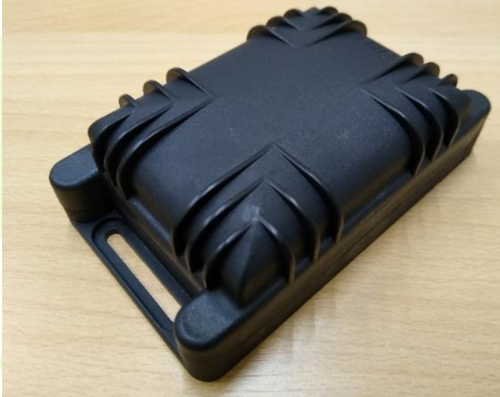
Abeeway Compact Tracker - GPS asset tracker converted to a livestock tracker
